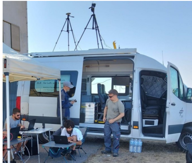
Figure 12: DLR-KN Ground Station. This image shows the mobile command van during field operations, highlighting its deployment capability and dedicated workspace.
