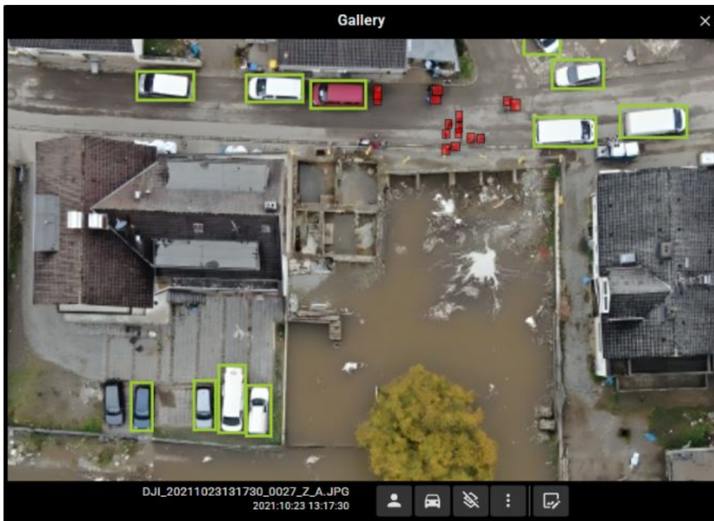
Figure 6. Person and Vehicle detection (TFA-tech-05).
