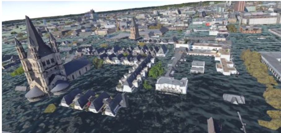
Figure 28. First prototype of the flood visualization using a simple water plane with adjustable height to demonstrate the concept.
