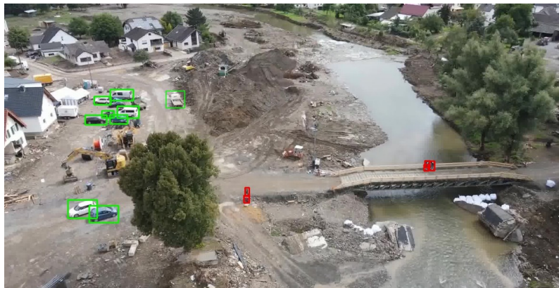
Figure 15. Person (red) and car (green) detection in the flooded Ahr valley, using RT-DETR-R18 [8] trained with the proposed method (LSB).
